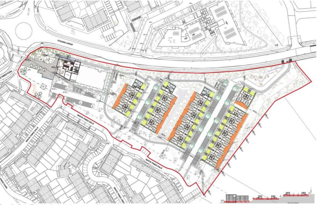
Figure 19 – Ground Floor plan with private patios, terraces and balconies to the apartment units
