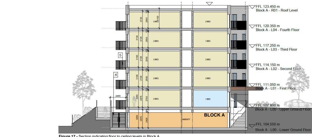
Figure 17 - Section indicating floor to ceiling levels in Block A
