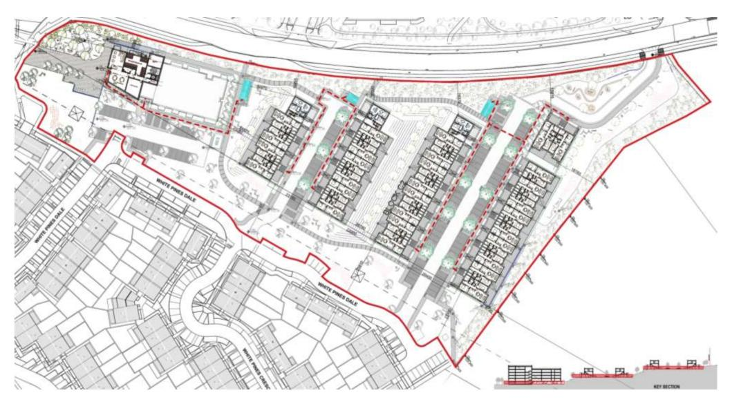
Figure 23 - Ground floor plan with waste storage locations and routes from dwellings to waste storage highlighted
